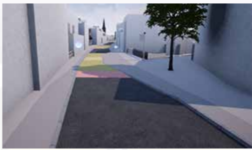
Raised table at buildout forming uncontrolled crossing
