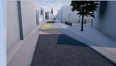
Raised table at buildout forming uncontrolled crossing
