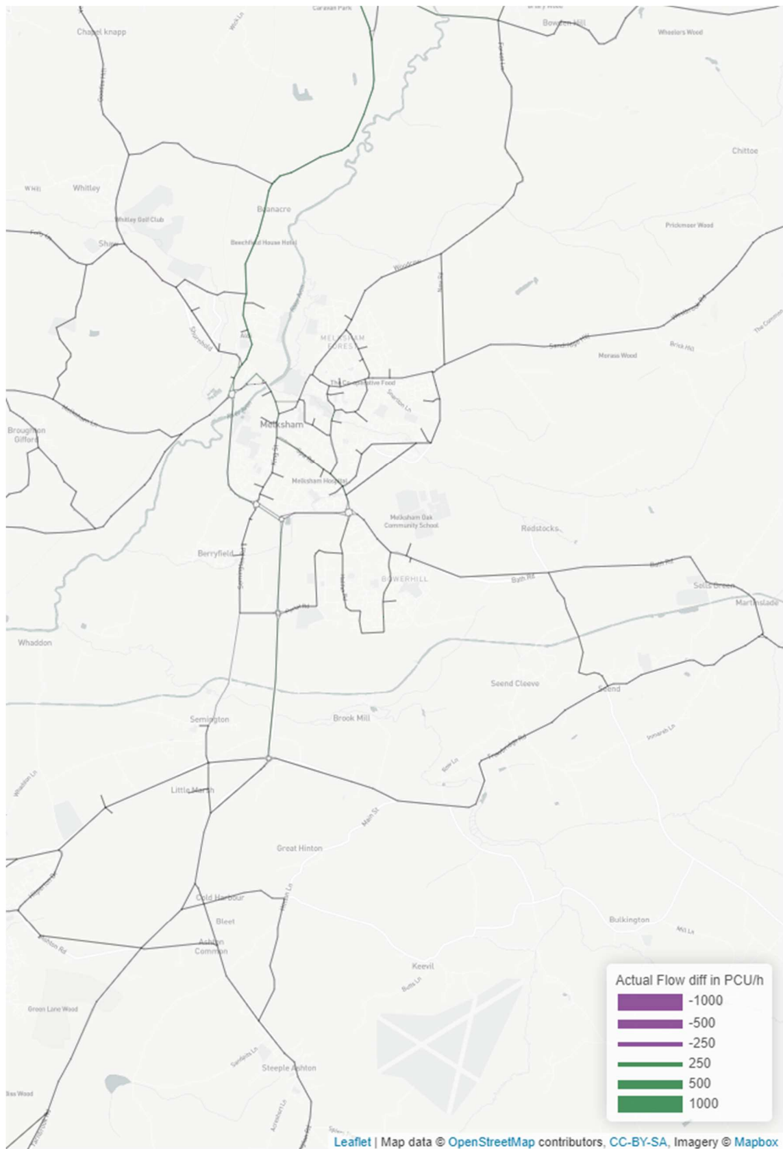
Figure H.7 - Difference in actual flow (PCUs): MRN DM - Core DM (2036 AM peak)
