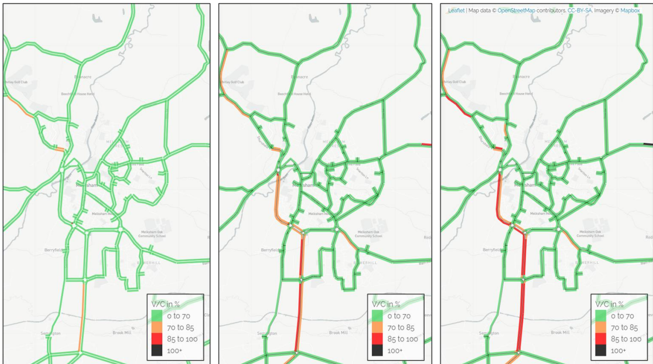
Figure 2-36 - Volume to capacity ratio for 2018 (left), 2036 (centre), and 2051 (right) - AM peak period (Wiltshire Transport Model)
