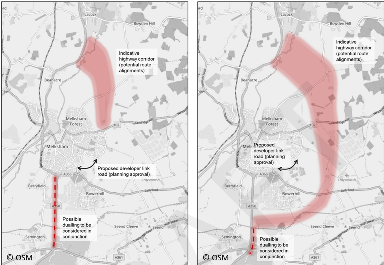
Figure 9-3 – Indicative corridors subject to further consideration of route alignments – option 10a (left) and 10c (right)
