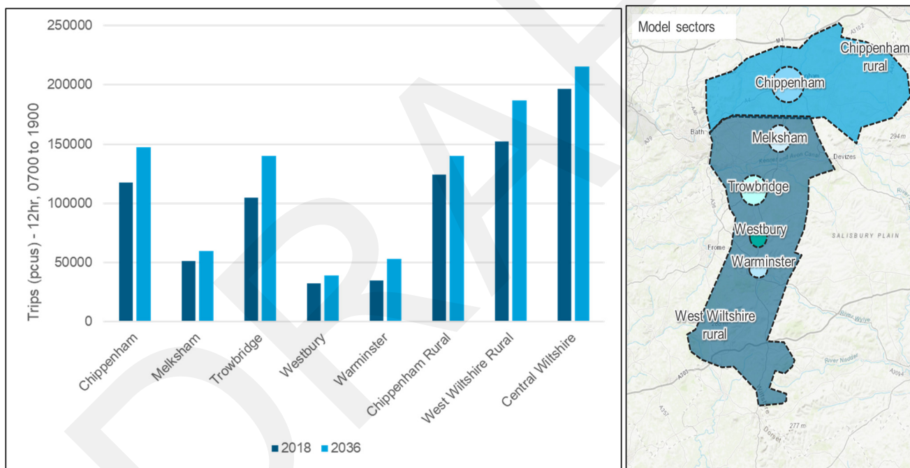
Figure 3-5 - Change in forecast 12-hr vehicle trip ends 2018-2036 (Wiltshire Transport Model, core growth scenario)
