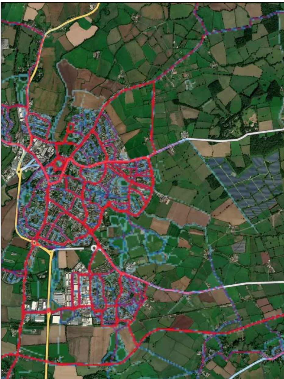
Figure 2-21 - Strava walking Heatmap for scheme extents (red – higher use, blue – low use)
