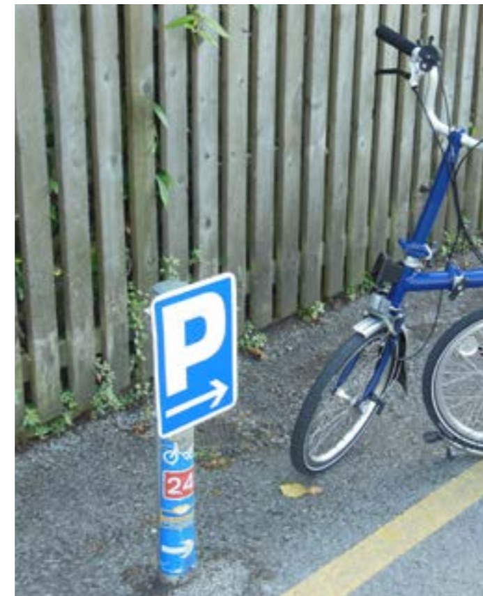
Low level signage is often appropriate for cycles and minimises the cluttering of streets with obtrusive tall poles.
