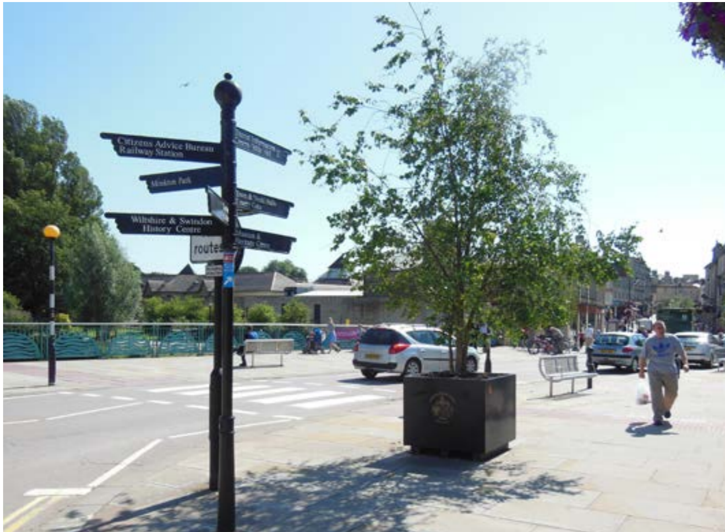
Appropriately placed fingerposts at key junctions enhance legibility for pedestrians and cyclists, although map based systems can provide more benefit in key locations. In this instance additional cycle route information was not integrated into the original design and has been positioned after installation.
